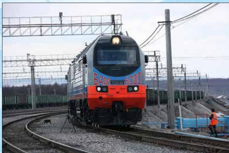
Coupled diesel locomotive 2TE25A Witiaz (Knight) with asynchronous traction drive on Baikal-Amur Railway Line (Russia)
