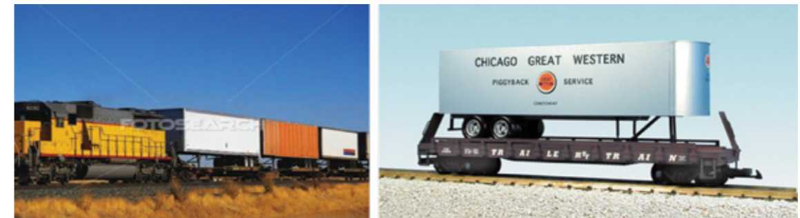
Fig. 22. Rolling stock used for piggyback transport
