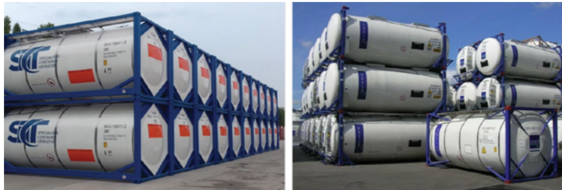
Fig. 43. Tank containers designed to transport various liquids and liquefied gases
