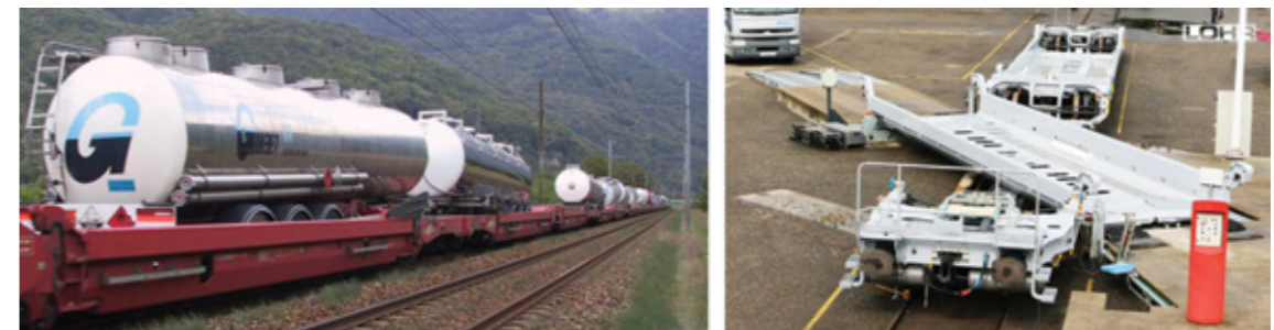
Fig. 5. Low-floor flatbed wagons used in piggyback transport
