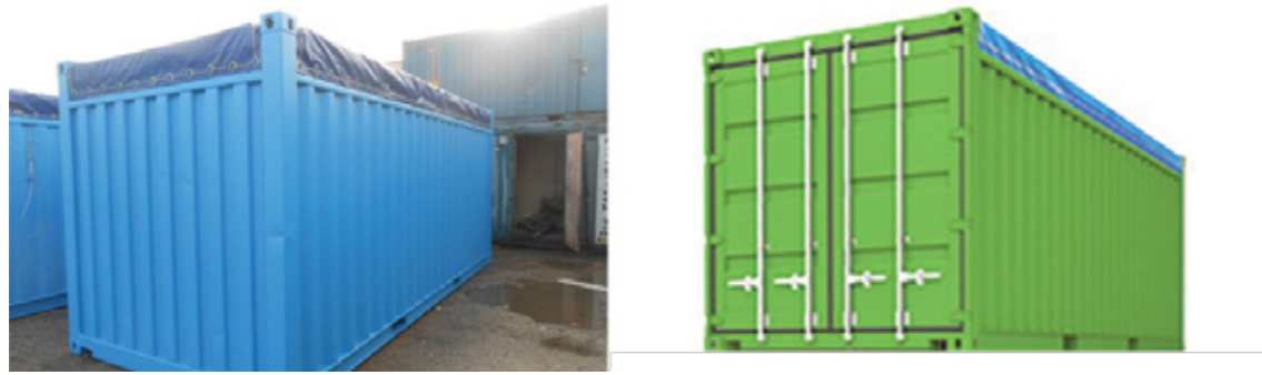
Fig. 48. Open top container
