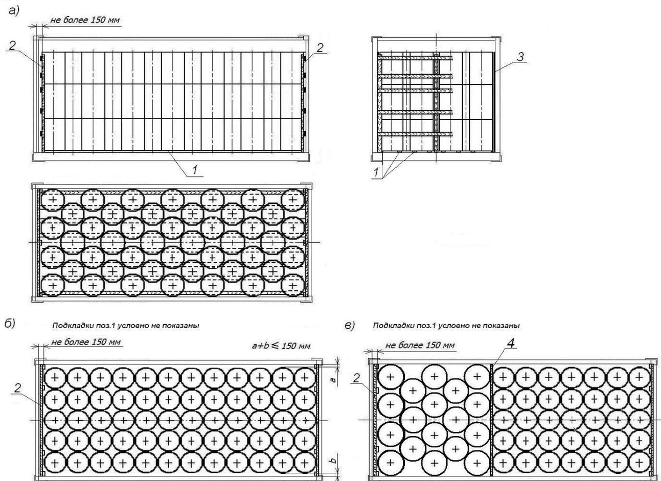
Figure 11 – Samples of stowing of cargo in a cylindrical package in a compact stack
