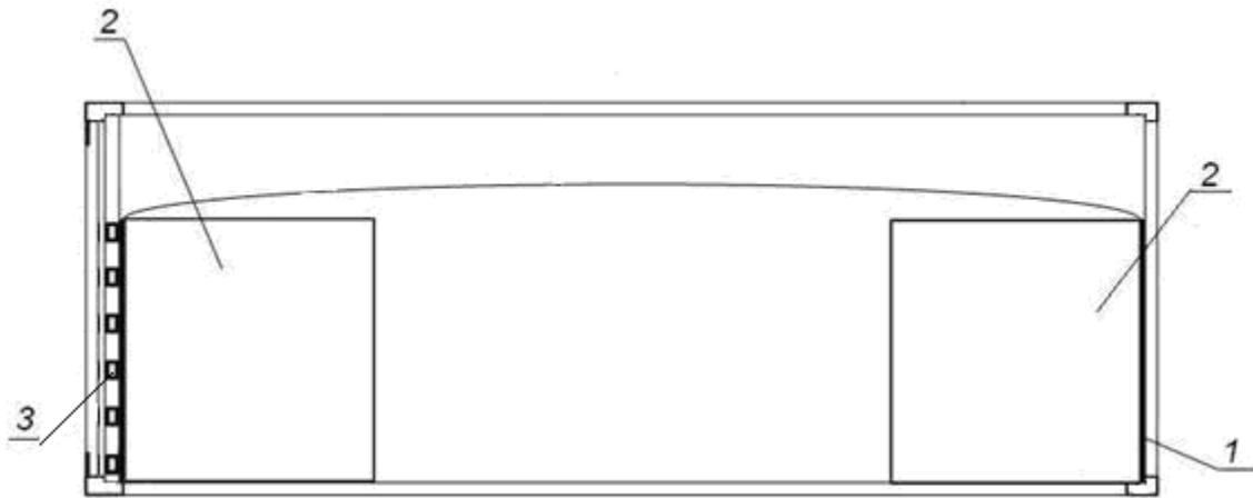
Figure 21 – Fastening of Flexitank in a container with grooves in corner posts
