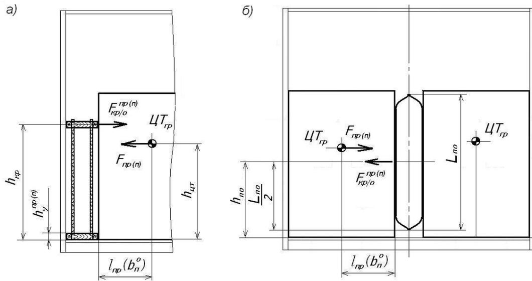
Figure 4 – Calculation scheme concerning the fastening of goods through
