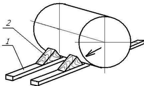
Figure 5 – Installation of wedges (blocking bars)
