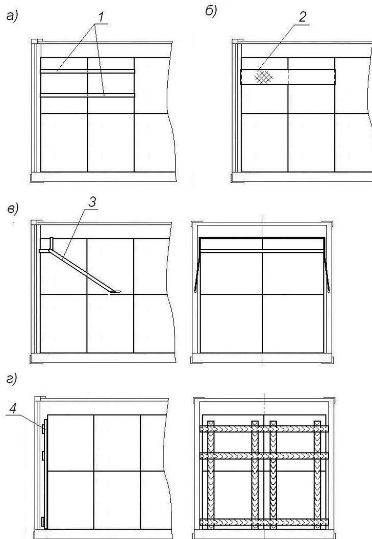
Figure 12 – Samples for ensuring load stability
