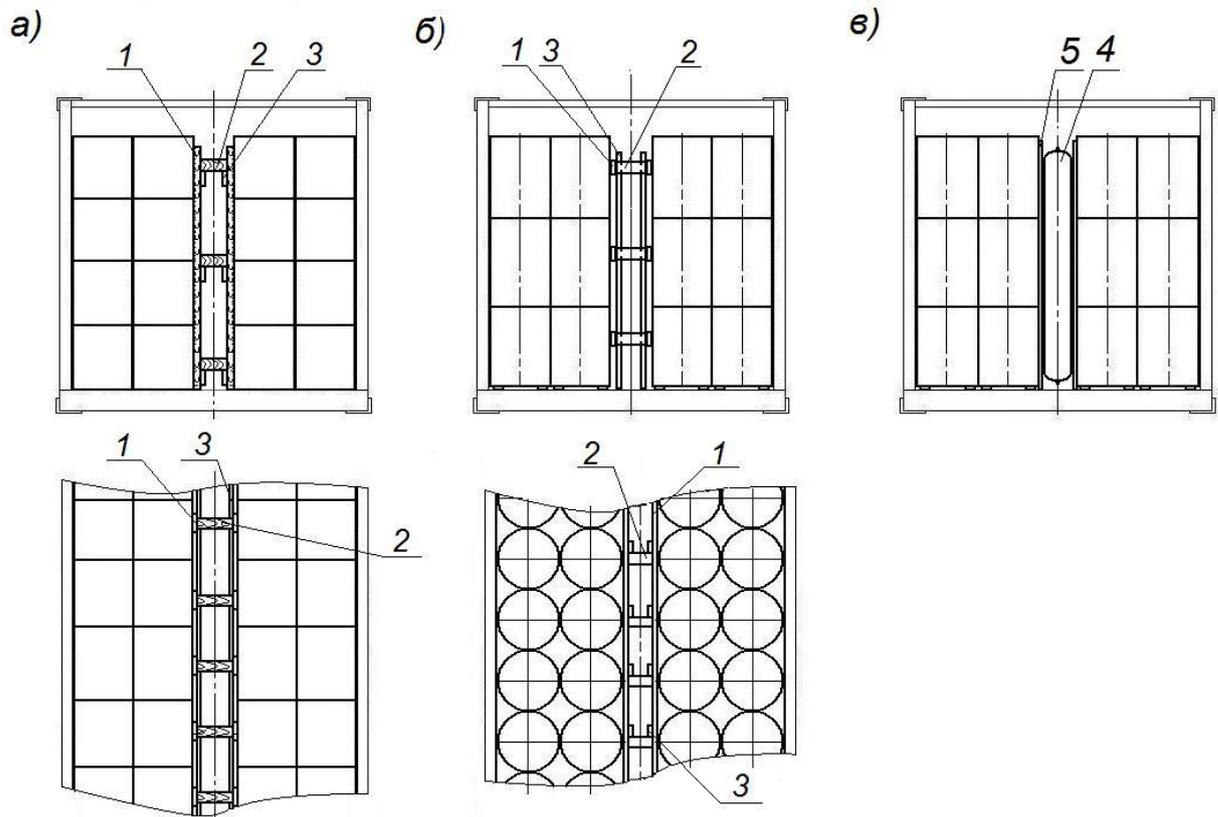
Рисунок 16 – A sample of fastening in lateral direction
