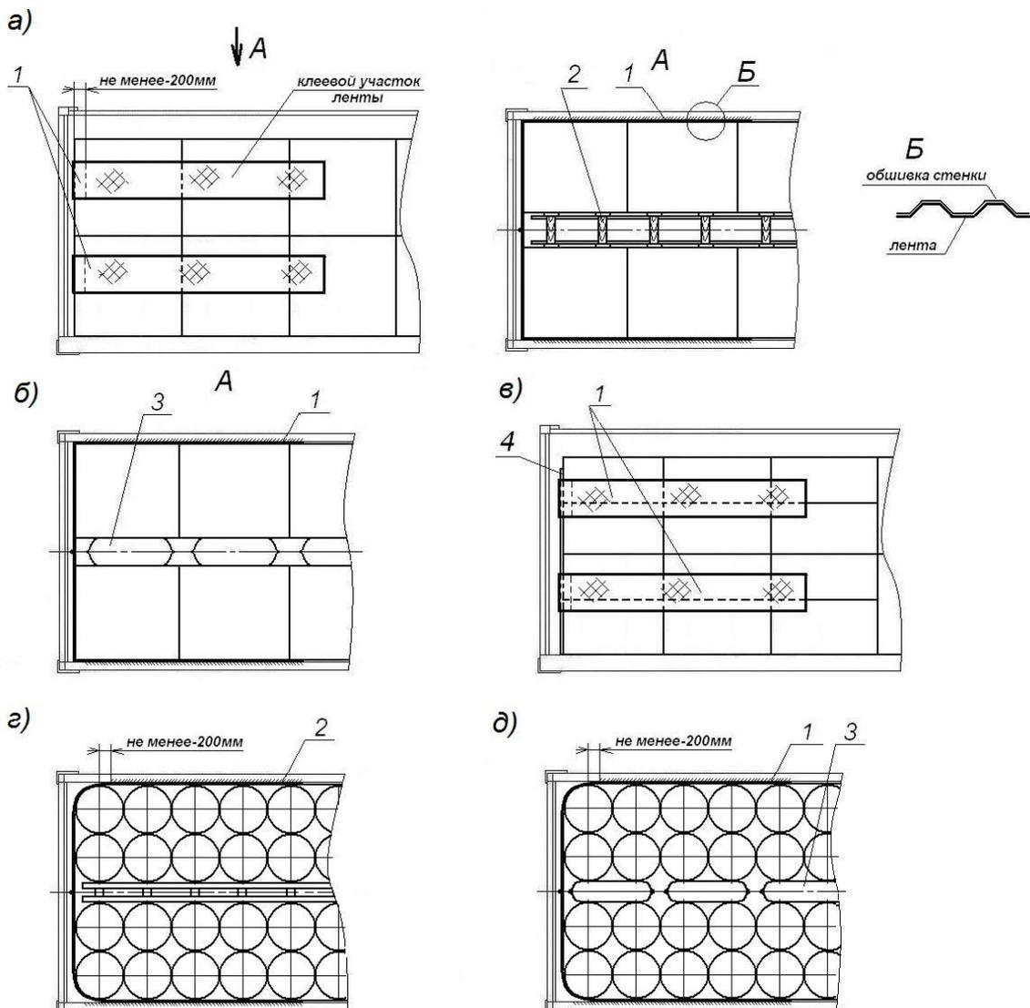
Рисунок 15 – Samples of fastening with a tiedown adhesive strip
