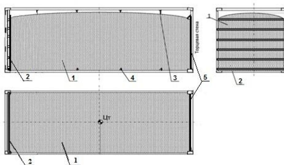
Figure 25 – Pattern of stowage and fastening of bulk goods using a liner
