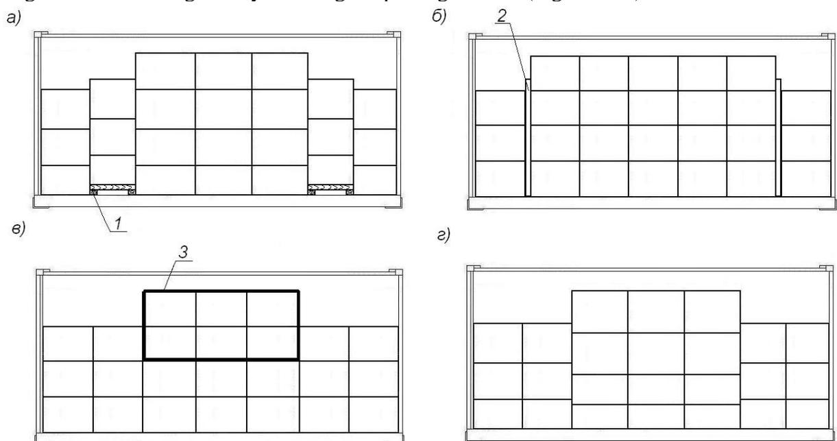
Figure 10 – Samples of cargo securing in an incomplete upper tier
