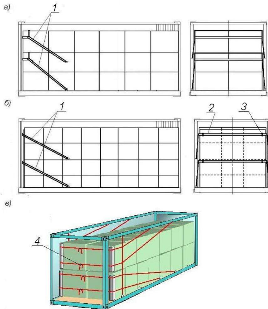
Figure 14 – A sample of fastening with straps
