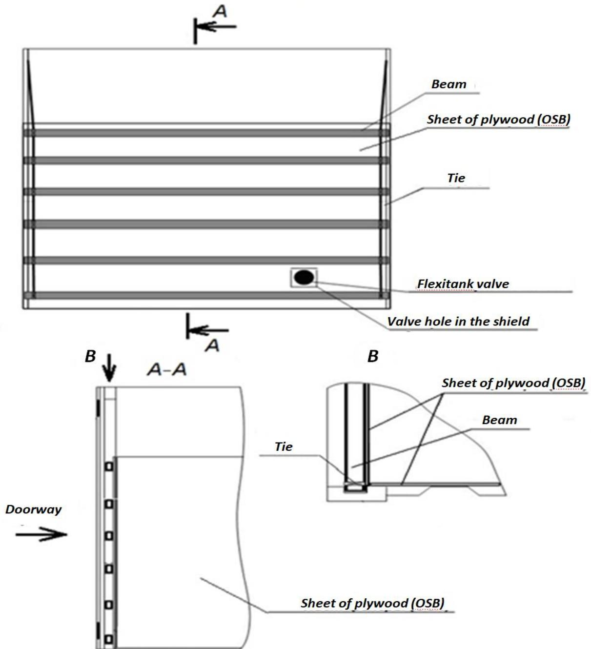
Figure 22 – Shielding of the doorway opening in a container with grooves in corner posts
