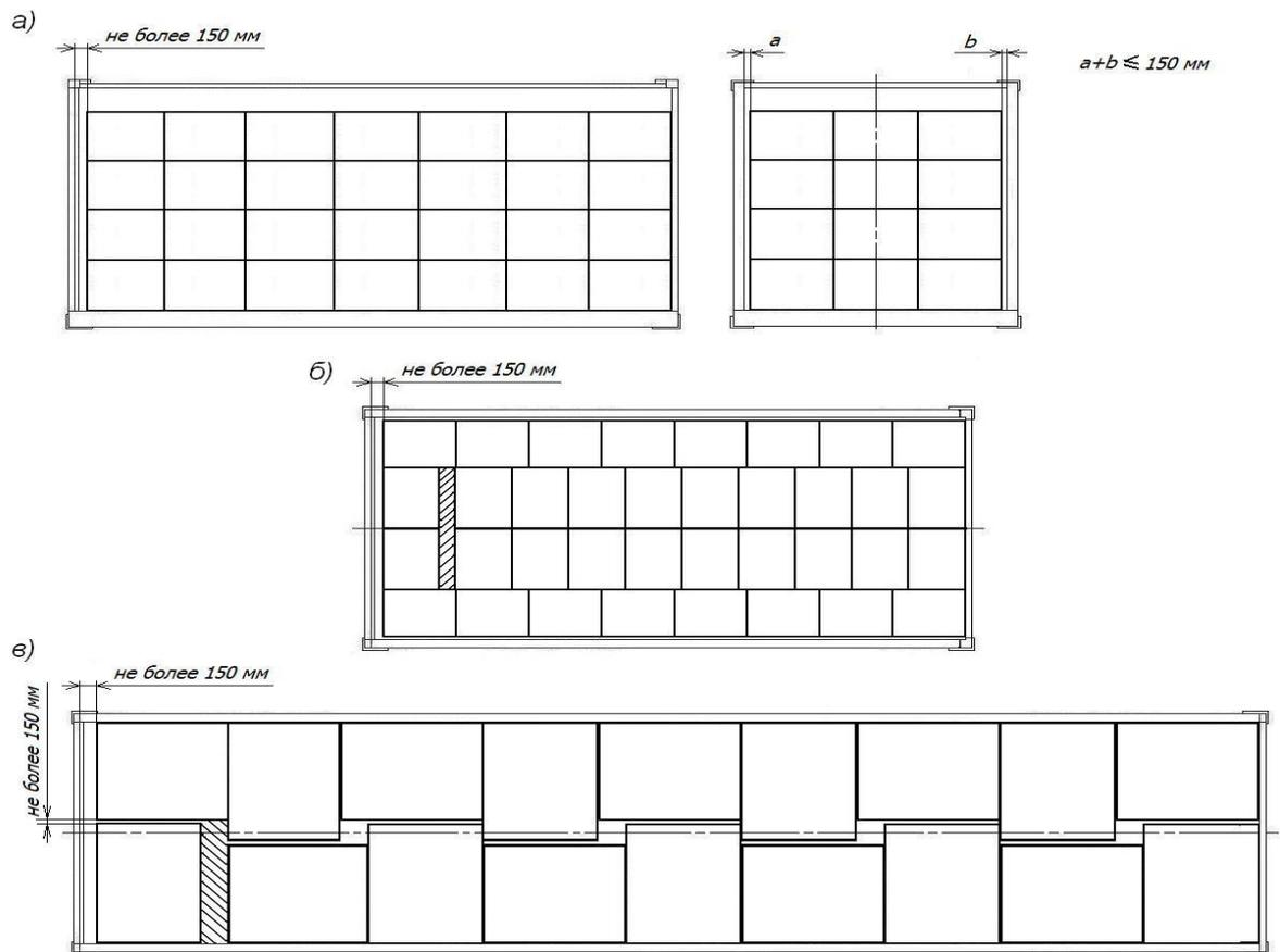
Figure 8 – Samples of stowage of cartons, boxes, packages in compact stack (the gaps to be filled are shaded, the end shield of the door fencing is conventionally not shown)
