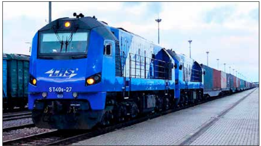
Container train which arrived in Poland from China without reloading goods at the EU border via the PKP LHS line with 1520-mm track gauge (07.01.2020, Sławków, Poland)
