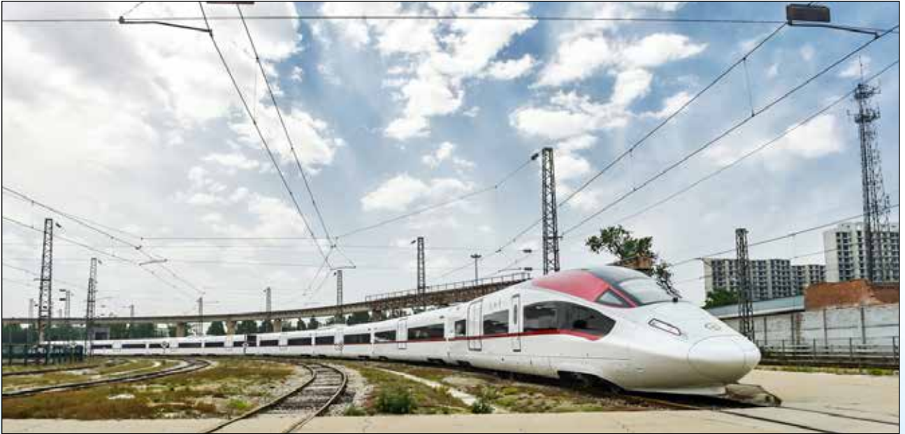
The high-speed train manufactured in China for the transportation of goods at a speed of 350 km/h
