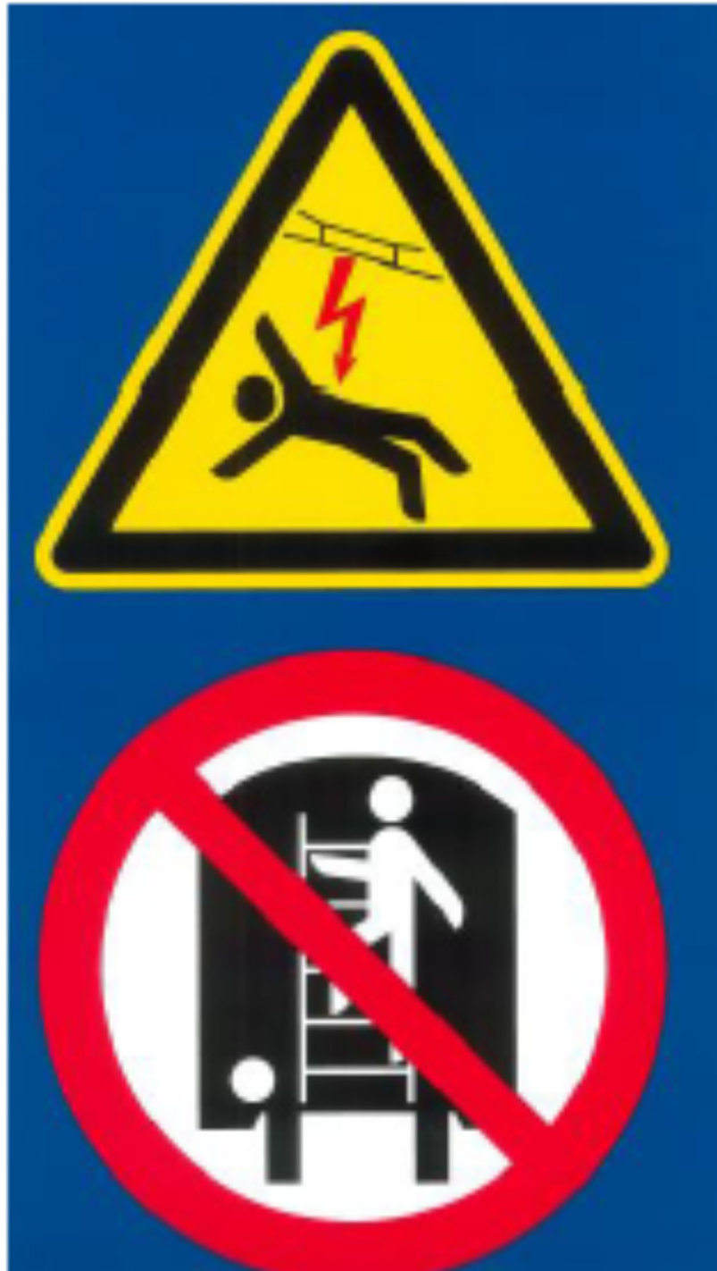
Fig.1.b. The sign to be affixed to wagons of 1435 mm track gauge.
