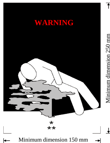
Asphyxiation warning mark for wagons and containers
