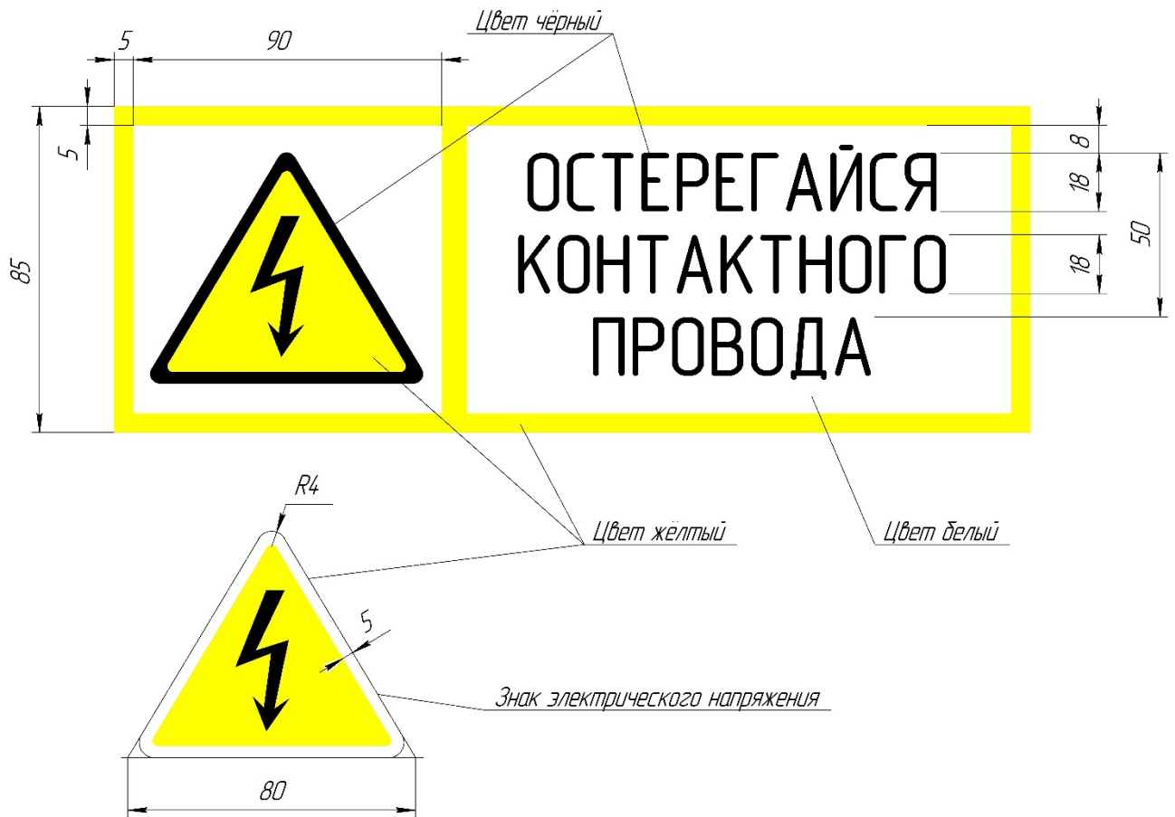
Figure 2. The sign to be affixed to wagons of 1520 mm gauge.
