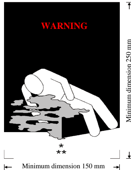
Asphyxiation warning mark for wagons and containers
